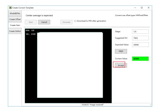
The gain template generation process needs 5 images total, the UI gives the recommended KV and target value, user can use different ones if needed.
