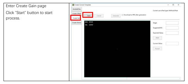
Click PREP button, acquire image. Please exposure after Acquire button enable. And click Acquire button to acquire image after exposure end. Click Accept button after acquired image. If Current Value textbox is yellow, click PREP button. Re-acquire images after adjust generator parameters.
