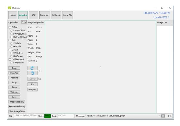
Status bar shows detector's serial number, the current task and state of detector, and feedback information of command. Status bar is also can be seen in other pages, and they are all the same.
