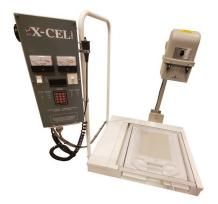
Example of older X-cel MB-700 modified with new 3.5"h SD Base and 1012V panel.
